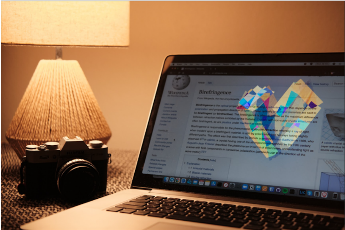
You see random cuts of tape stuck on the screen in the shape of a heart through a linear polariser. Plastic molecules are elongated thus the tape exhibits birefringence properties. Ordinary and extraordinary rays may exit the plastic in or out of phase depending on wavelength and thickness resulting in a colourful image. Photo by Ivan Toftul.
