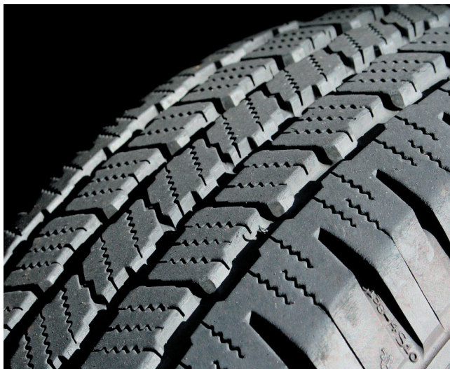
Groovy tread: a Michelin tyre showing the radial and transverse grooves that form the tread. (Courtesy: Scott Robinson/CC BY 2.0)
