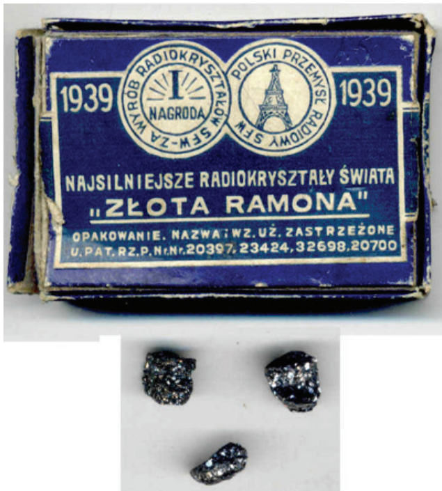
Figure 4: Crystals of Galena (lead sulphide) used for receiving radio transmission in Poland in 1939 [4].
