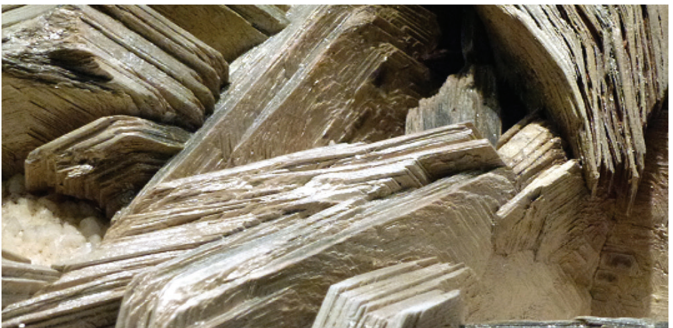
Figure 5: Structure of mica, showing the thin sheets of crystals which give this complex mineral its space-age properties [5].
